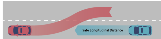
Figure 13(b): safe cut-in as the red car is not violating the frontal longitudinal safe distance of the blue car
